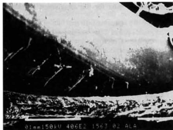
Fig. 9. Scanning electron micrograph of one of the \{210\} side faces of ( R,S )-alanine etched by ( S )-threonine; only two adjoining faces are shown, one etched and the other smooth.
